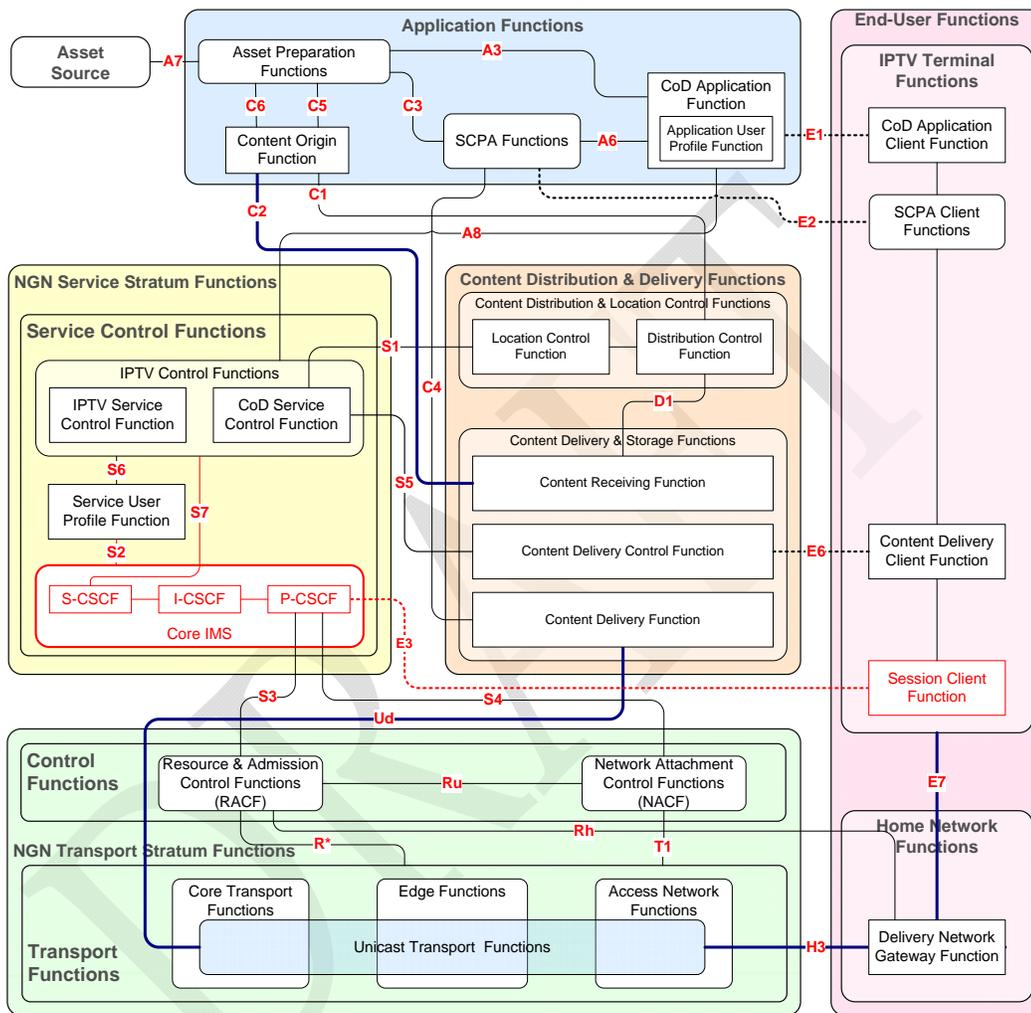
Figure 3: Functional Architecture for IMS CoD
