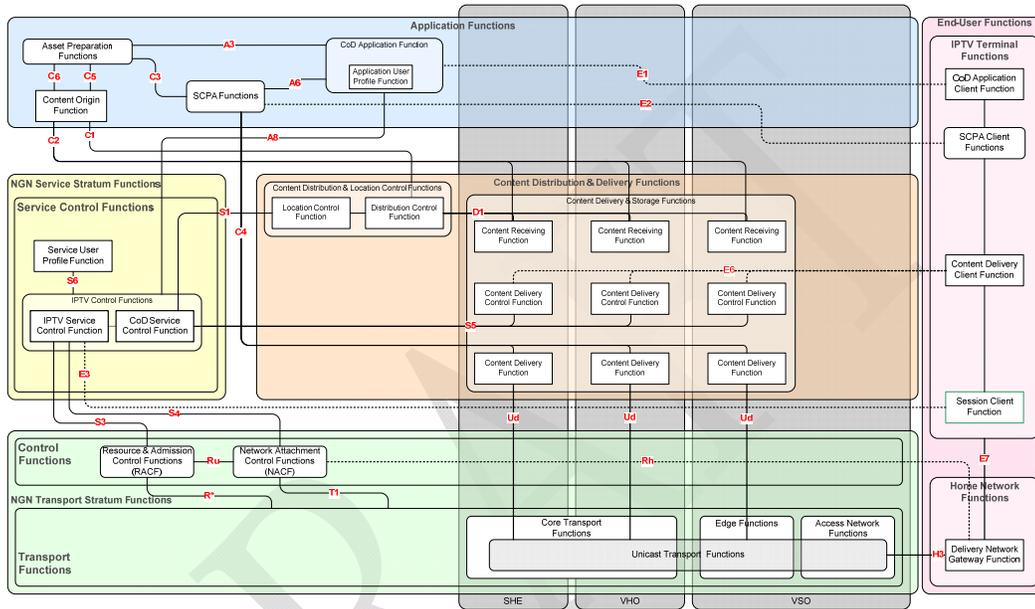
Figure 4: Geographically Distributed Functional Architecture for non-IMS CoD
