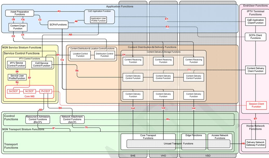
**Figure 5: Geographically Distributed Functional Architecture for IMS CoD**
