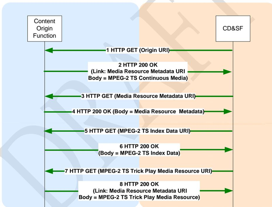
Figure 27: MPEG-2 TS Media Resource Prepositioning Flow
