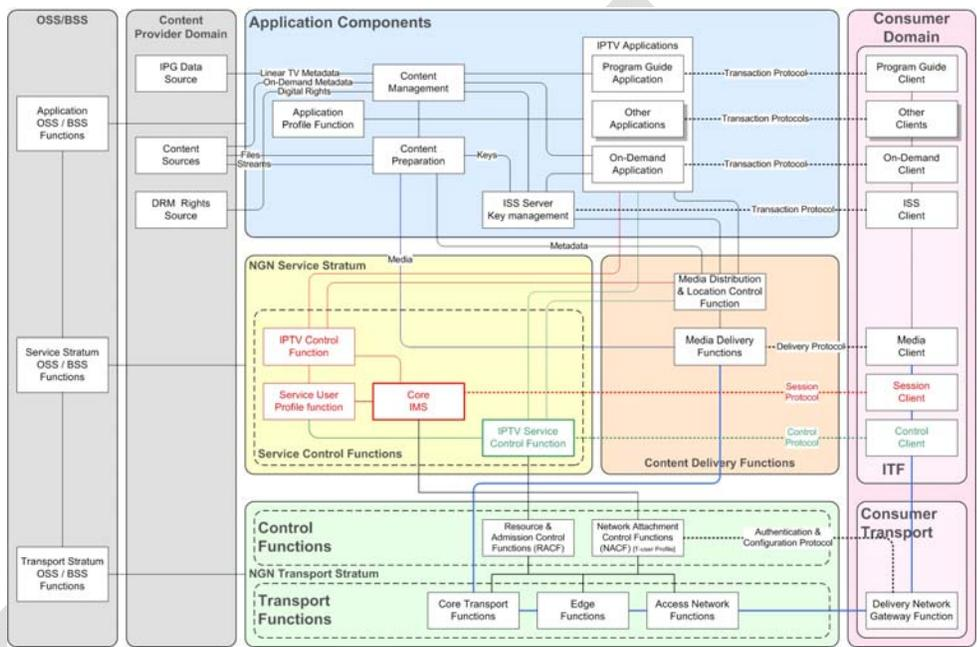
Figure 1: IPTV High Level Architecture
