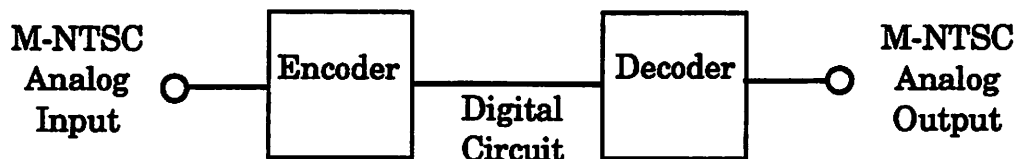
Figure 1 Digital Transmission Service Channel with Interfaces
