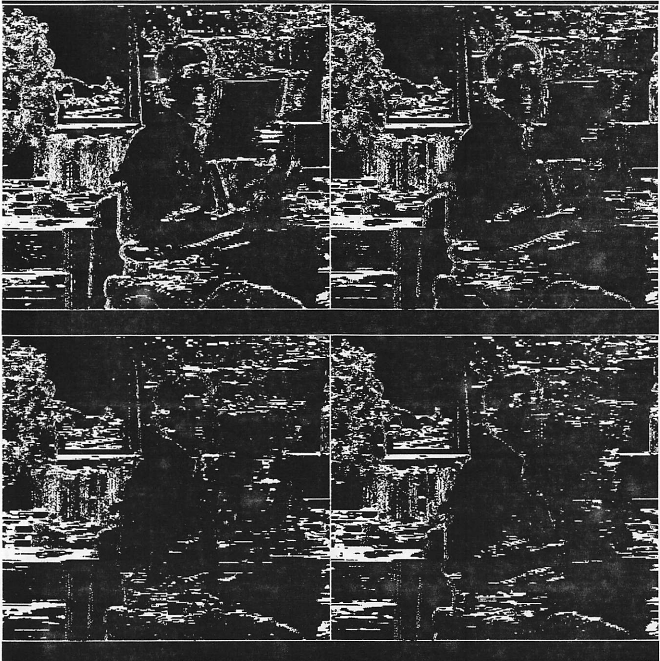
Fig. 2b. Median filtered (3x3) & Laplacian (3x3) edge detected binary images of Fig. 1 (From upper left clockwise: NTSC, T1, 1/2T1, 1/4T1).
