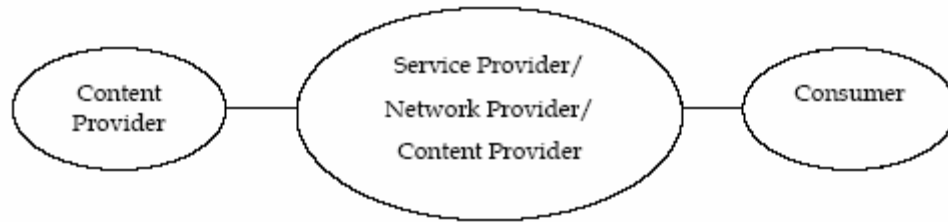
Figure 3: One Provider Implementing Multiple Providing Roles
