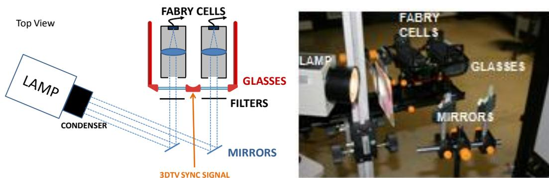
Figure 3 – Set-up for glasses measurement.
