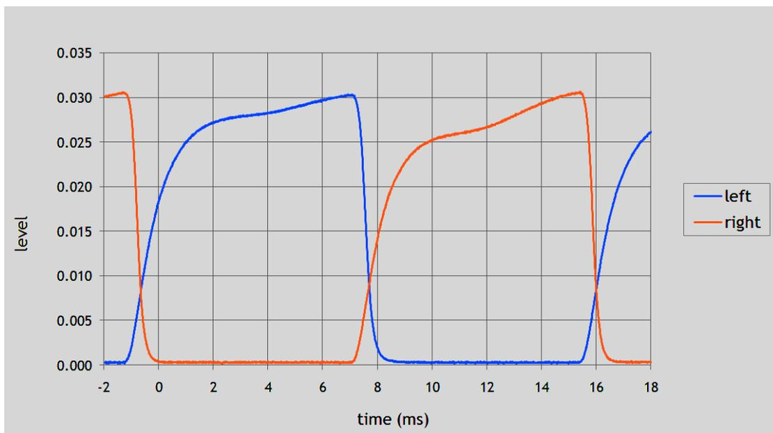
Figure 4 - Temporal measurement of glasses.
