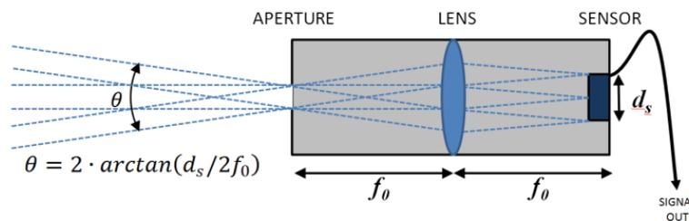
Figure 2 – Fabry assembly optical arrangement.
