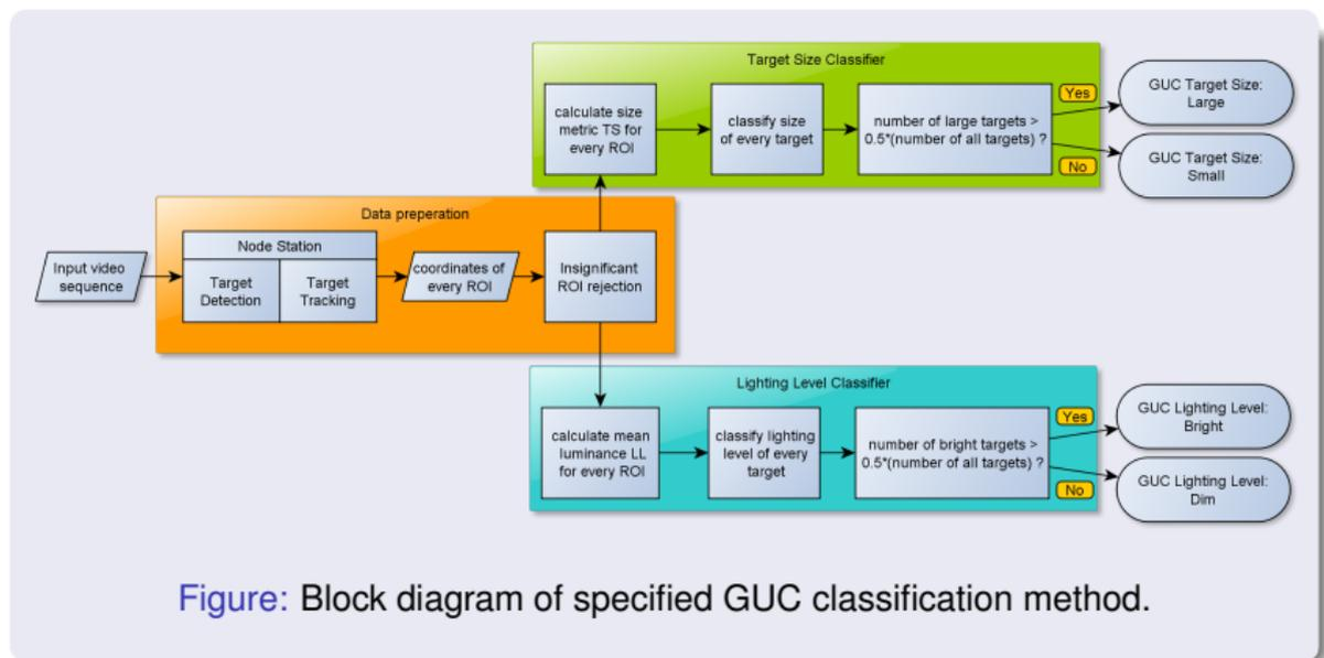
Figure: Block diagram of specified GUC classification method.
